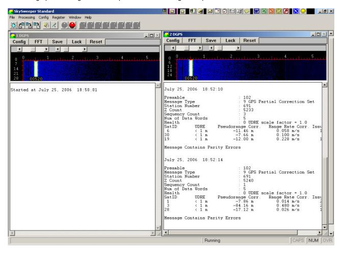
**Above:** The left-hand window is set to decode 200bps signals, the right hand one is set for 100bps. In this example the Wormleighton beacon in the UK on 291.0 kHz has its 100bps signal decoded in the right-hand window, whereas if a 200bps signal was tuned in the left-hand window would start decoding instead. Note how the 3D config box and the Configuration Editor boxes have been turned off in this set up, and this gives a much cleaner working area for the user.
