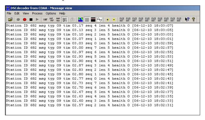
As you can see in the data above, the message window displays the Beacon ID, followed by the Message Type, which are the main items that DGPS DXers are interested in, and at the right-hand side of the screen we can see the date and time that the message was received (in this case this is in yy/mm/dd format, or the
