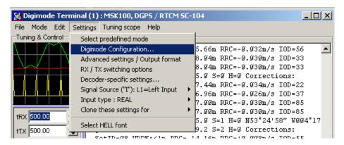
To change the baud rate, bring up the 'Digimode Configuration' window and then change the 'Symbol Rate; Baudrate' setting as shown below from 100 to 200 as required. Click 'OK' to remove the window again.
