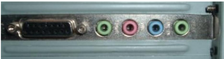
You can see that there are four 'jack' sockets here, though some cards will often just have three. In this case the Pink socket is for a microphone, the blue one is the Line Input, and green is for the speakers.
