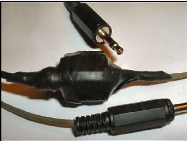
**Above:** *the final assembly, wrapped in self- amalgamating tape for extra strength and insulation!*
