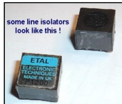
Above left is a picture of an old 56k modem showing the line isolation transformer, and above right we can see some other examples of the types of filters you might encounter on these boards. These two types are the ones I've usually encountered, but there may be other types that look slightly different on boards from other countries.
